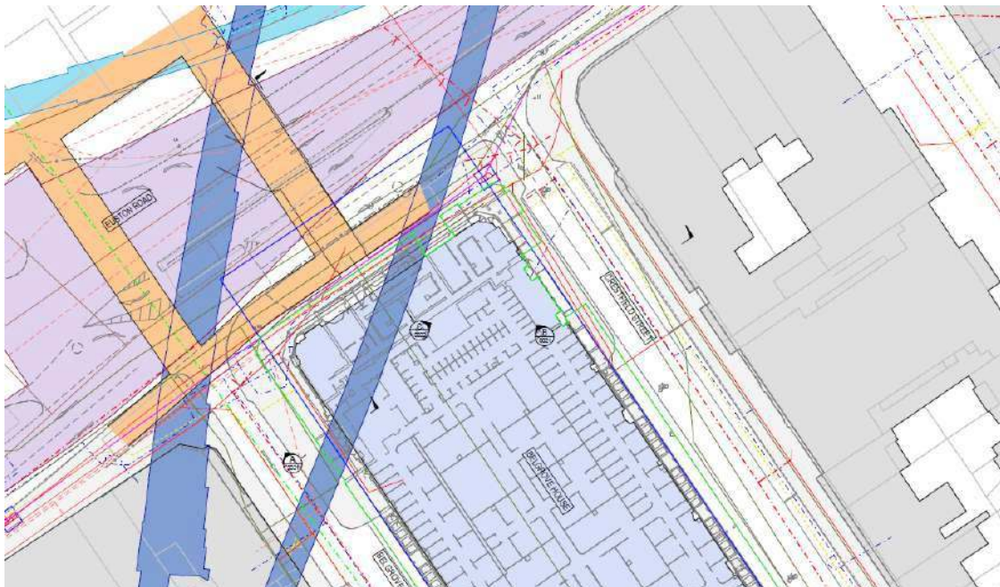
Extract of site constraint plan indicating location of Piccadilly Line tunnels and Kings Cross station entrance tunnels
