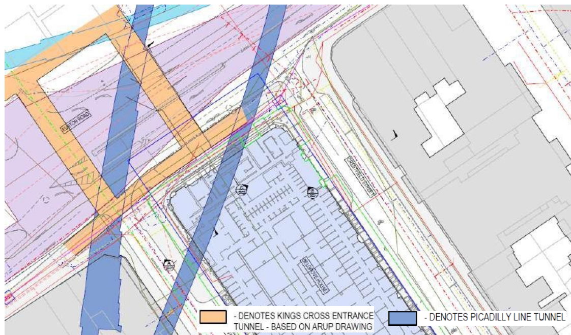
Figure 09 – Extract of site constraint plan indicating location of Piccadilly Line tunnels and Kings Cross station entrance tunnels
