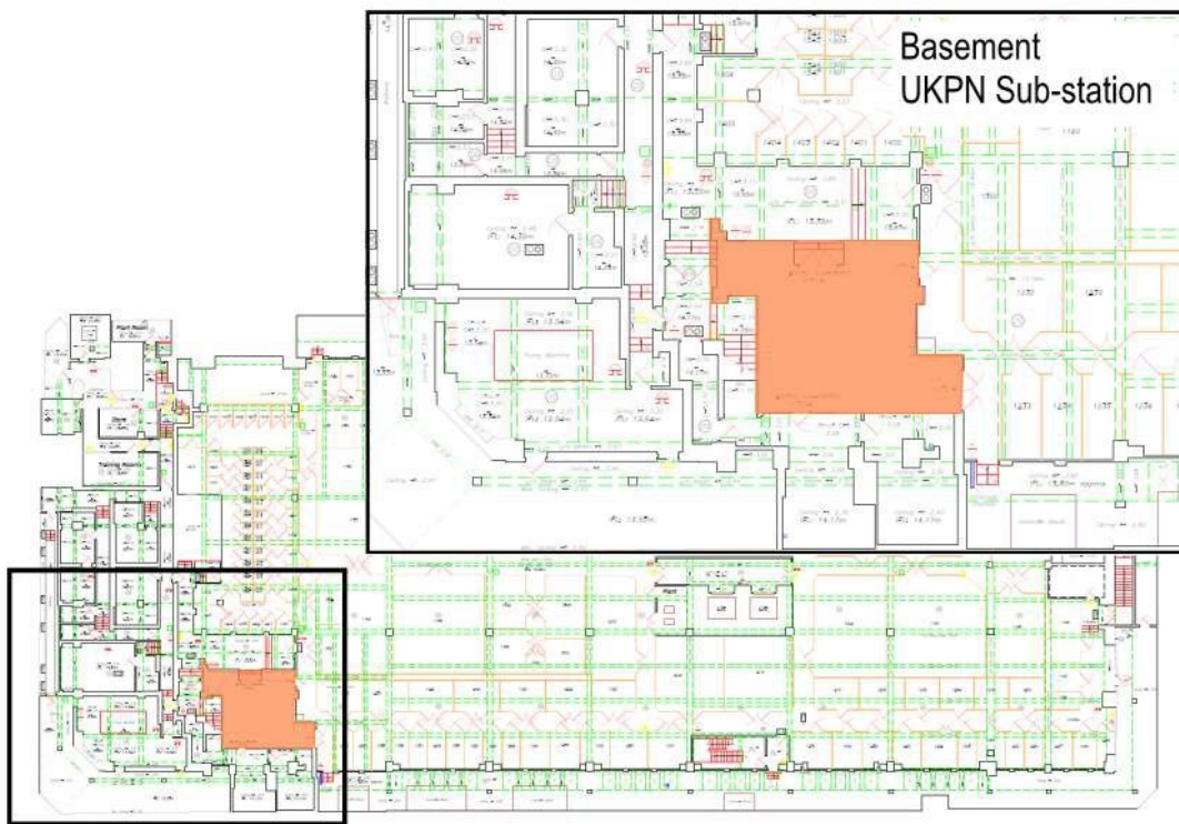
Figure 04 – Extract of UKPN plan denoting existing sub-station
